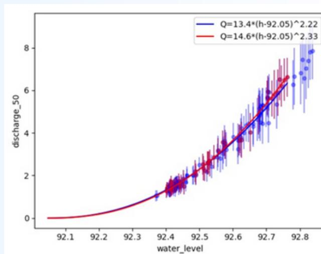
Figure 10. Rating curve after one month of measurements
