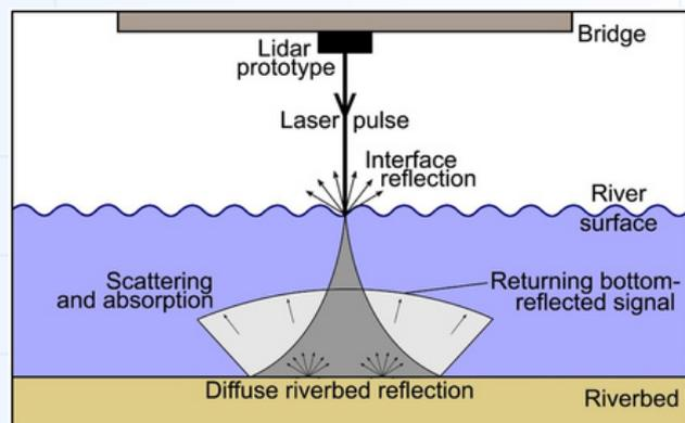
Figure 3. Schematic of lidar water level sensor illustrating the fate of laser pulses (Paul et al. 2020)
