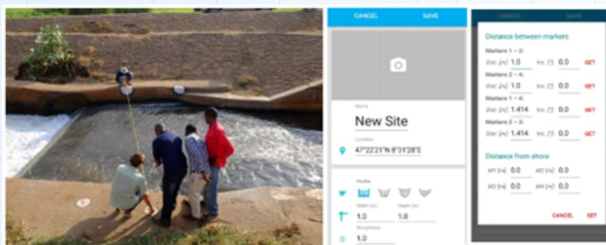
Figure 12. Site setup for the DischargeApp
