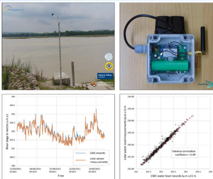
Figure 4. (Anticlockwise from top-left) River bank installation of lidar water level sensor at Haridwar on the River Ganga, India; Time series of river stage observations at Haridwar on the River Ganga; Pair-wise scatter plot between Central Water Commission (CWC) gauge records and lidar water level sensor readings; the low-cost lidar water level sensor developed for the WMO HydroHub Second Innovation Call.
