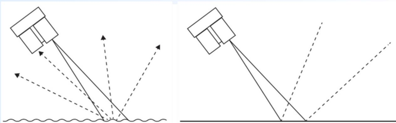
Figure 1. (left) Diffuse reflective surface; (right) Specular reflective surface (Source: Garmin Lidar Lite v3 manual)
